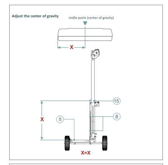
Determine the center of gravity for roof tents with an asymmetrical structure or equipment.
